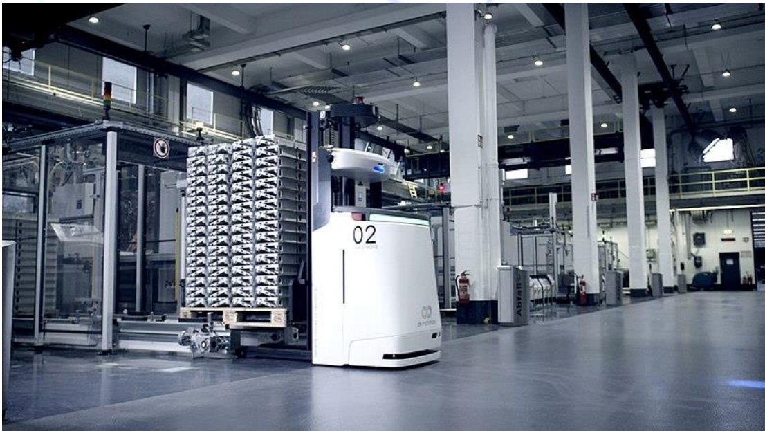
Figure 5: An automated guided vehicle (picture by ek robotics GmbH, licensed under CC BY-SA 4.0)
