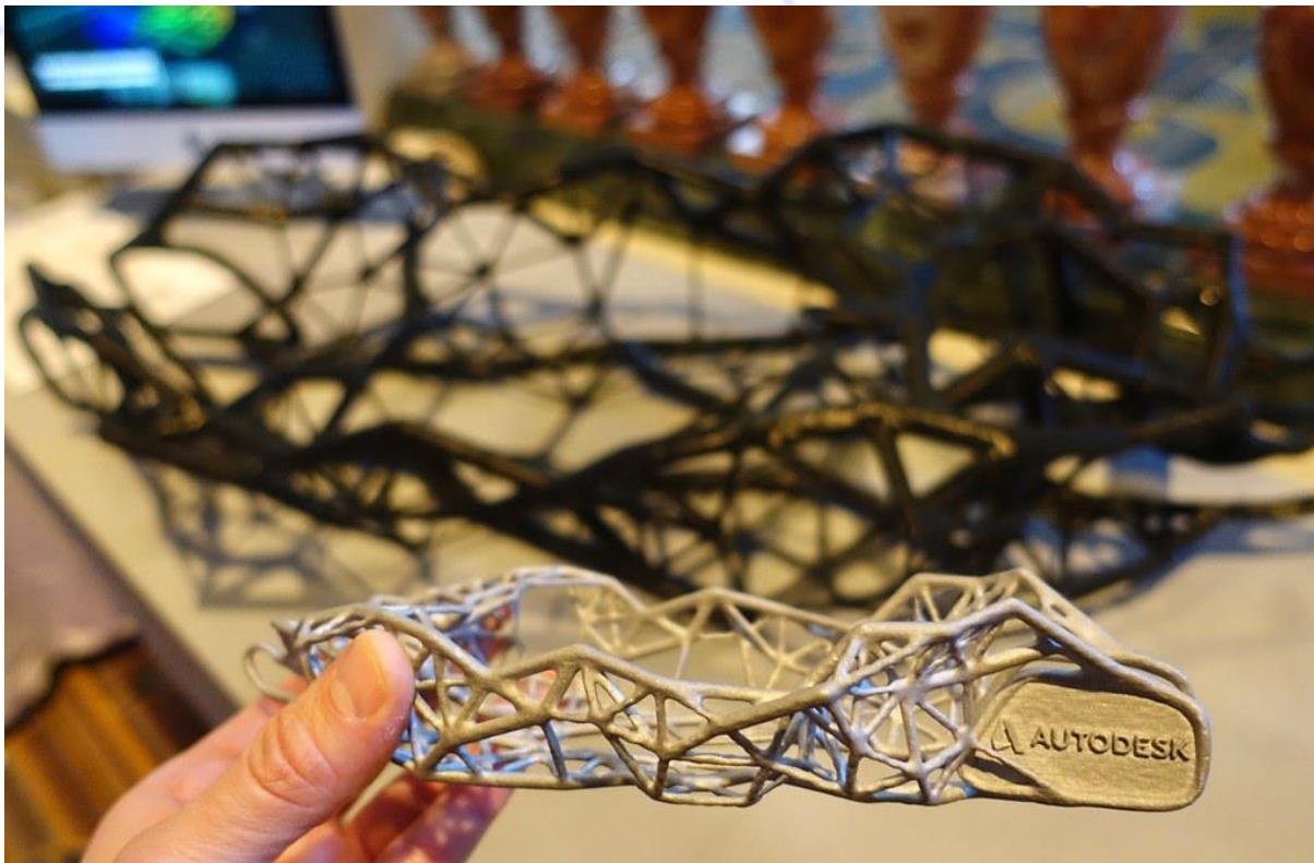
Figure 8: Generative design model of a car chassis (picture by Steve Jurvetson, licensed under CC BY 2.0)
